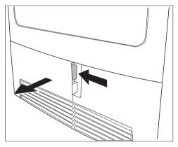
Open door in plinth: To do this, press the release button on the right and open the door in the plinth to the left.
